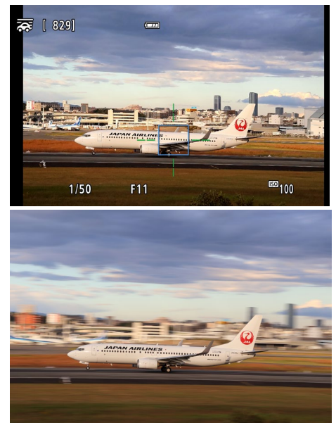
Subject Blur Guide is a new feature on the EOS R50. Track the horizontal green line with the camera and the R50 optimises settings for better panning shots.
